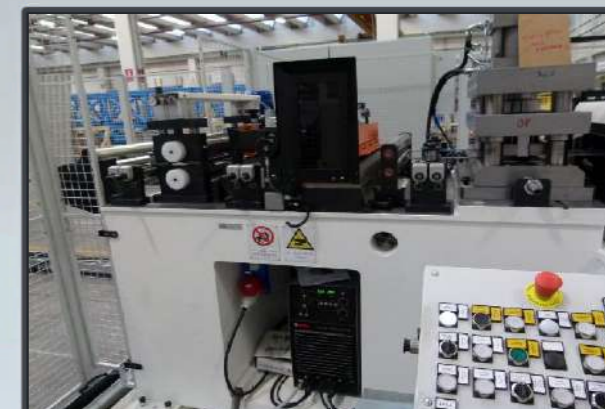
Welding and heading bench
