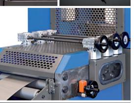
**Despite having a working power of 20 Tons, OROBIA is the entry level machine of the punching lines realized by Produtech.** It is an economic, simple and rapid machine characterized by a maximum working width of 400mm, the tools are not indexed.
